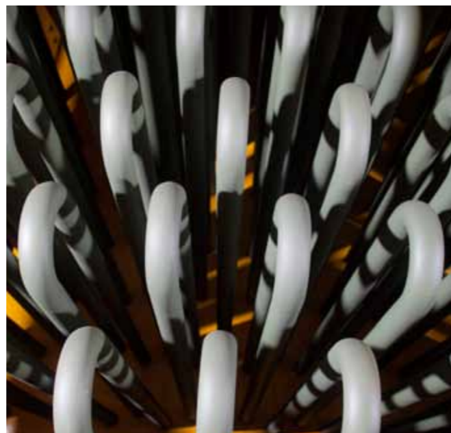
Passive cooling system qualified for the inlet and antisurge cooling of the process stream for the Ormen Lange Pilot compressor system
