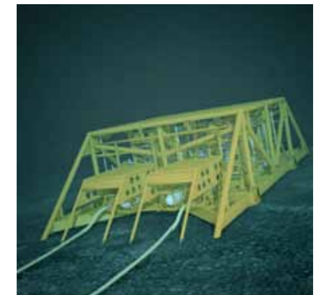
Subsea compression station with two compressor trains
