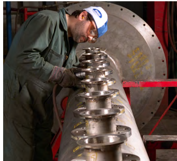
> SARAMET® piping distributor during fabrication
