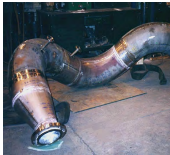
> SARAMET® pipe spool illustrating the benefits of welded construction by elimination of 7 flanged joints
