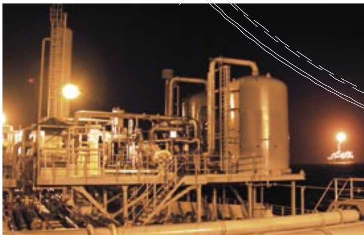
Marine based crude oil VRU on M/T Navion Europa
