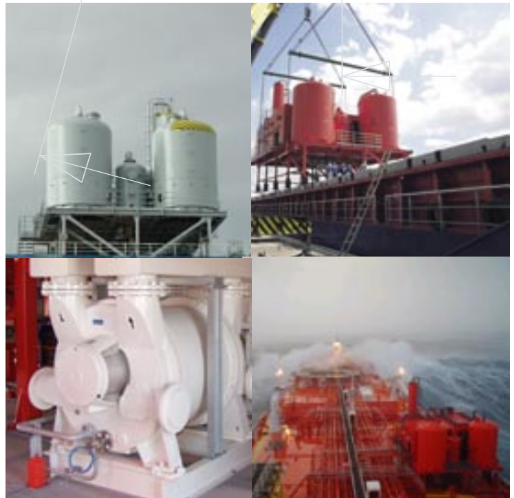
Top: Complete marine based VRUs. Bottom left: Vacuum pump of a marine based VRU. Bottom right: The Statoil shuttle tanker, Åsgard C, with its Aker Kvaerner Cool Sorption VRU in full operation during a heavy storm (picture courtesy of Statoil)
