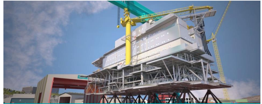
Johan Sverdrup utility and living quarters topside
